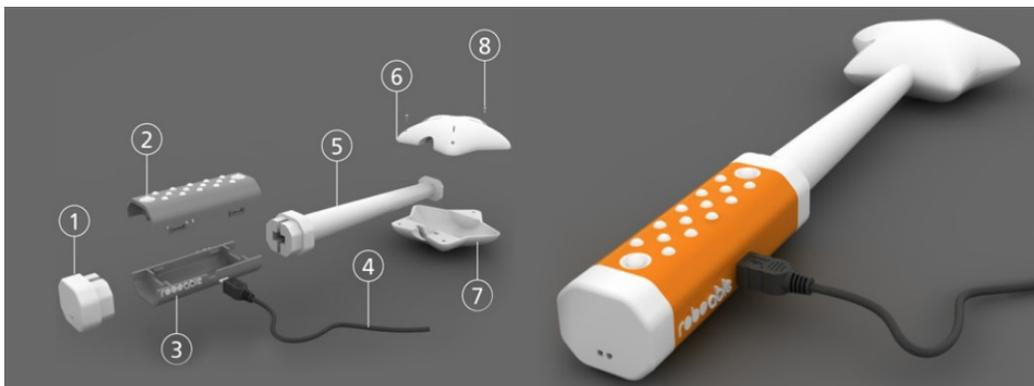
Figure 2. Roboable exploded.
